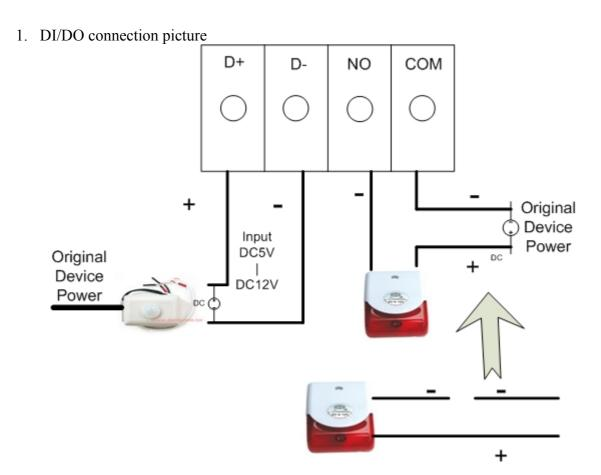
2. DI need a sensor can output a DC voltage between 5V-12V. For example we are use a sensor can output DC12V
